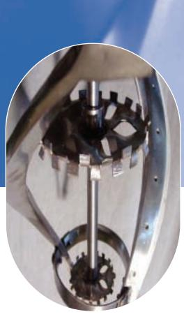
The **SC Mixer** is ideally suited for mixing or drying applications that require *finite control of reaction kinetics*. With either adjustable or high sheer capabilities, this mixer routinely handles materials with a viscosity as high as 3 million Centipoise.
